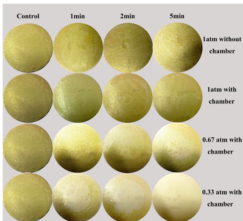
Figure 4. Anti-bacterial effect under different pressure with an applied voltage of 3 kV. The images show bacteria grown on nitrocellulose (NC) membrane surfaces after different times of plasma exposure. The top row is for a 1 atm application without a confining chamber. The near breakdown threshold applied voltage of 3 kV shows little antibacterial effect at 1 atm, but increasing effects at the lower pressures.
